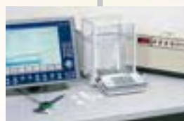
Testplace module with weighing station, tablet tester and dimension measurement
